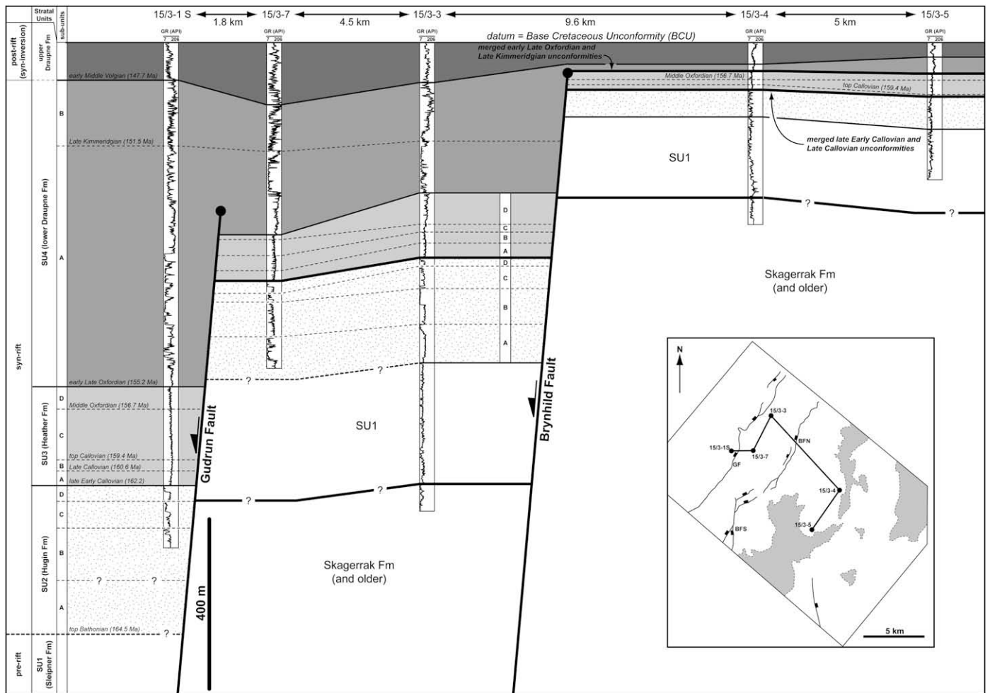
Fig. 6. Stratigraphic correlation of key wells within the study area illustrating thickness variations in the studied syn-rift stratal units (SU). The tectono-stratigraphic significance of the various syn-rift stratal units is indicated in the column of the left-hand side, as are the identified stratal sub-units (A, B, C, etc). The line of section is shown on the inset map; this is a simplified syn-rift structure map based on the top-SU2 (top Hugin Fm) time-structure map (see Fig. 3B). Thick solid black lines represent regionally mappable, stratal unit-bounding surfaces; thin dashed lines represent locally identified stratal surfaces which define sub-units; very thick black lines represent unconformities. GR = Gamma-ray. Note the thickening of SU1 (Sleipner Fm) and SU2 (Hugin Fm) across the Brynhild Fault is apparent, and is related to overall NW-thickening of these units rather than abrupt thickening across the fault.
